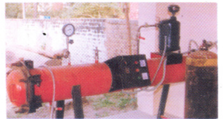
Ammonia Fumigation Plant
