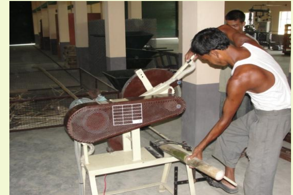
A view of newly established BCC - Cross Cutter and other advanced equipments
